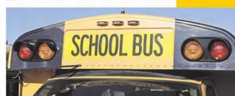
The additional amber lights are intended to warn motorists that buses are about to stop.
