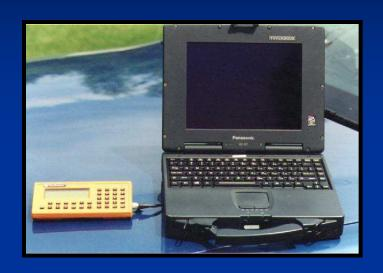
Total Station data collector is connected to a laptop computer, where recorded measurements are retrieved.
